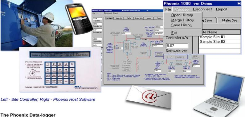
Monitoring includes data reporting on engine vital signs and system operation. Reports are generated automatically or manually at the discretion of the operator. Data is stored at programmable intervals for future retrieval, and it can be downloaded via direct or modem connection to the PC.
