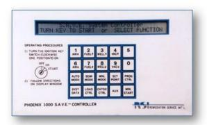
Critical to our success has been the development of the patented Phoenix S.A.V.E.™ Controller. It continuously monitors system operation to optimize system performance. The controller records process information for future retrieval and the telemetry feature allows bidirectional communication and control of the S.A.V.E.™ systems. These features significantly reduce labor costs associated with the operation of conventional remediation systems.
